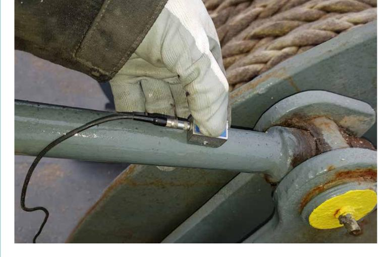
>> Ultrasonic testing This method will provide indications of surface and subsurface discontinuities, will determine by the use of the proper technique the depth and exact size of the damage in the material. Ultrasonic pulses are directed into the test object which produces echoes and reflections which then indicate the presence, absence and location of flaws, interface and/or discontinuities.
